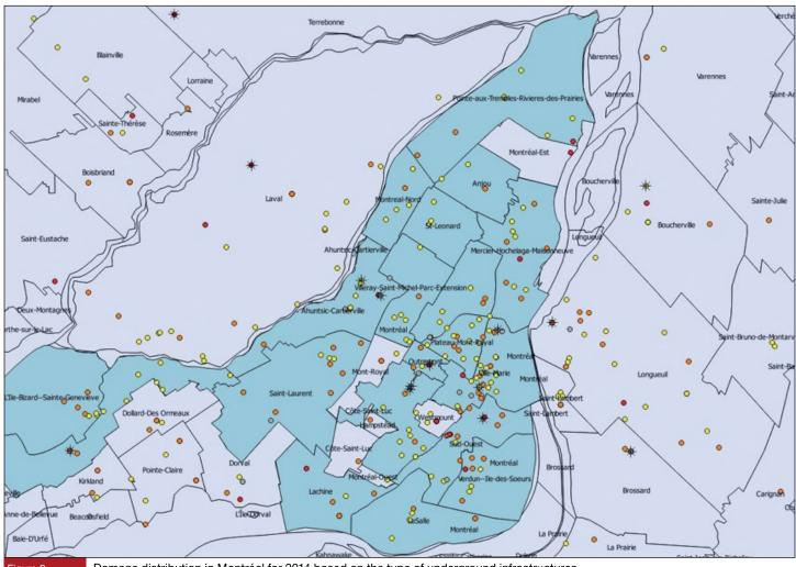
Figure 2 Damage distribution in Montréal for 2014 based on the type of underground infrastructures (Gas = Yellow ; Telecommunication = Orange ; Electricity = Red ; Others = Grey ; Star = Service interruptions of 5 hours or more)
